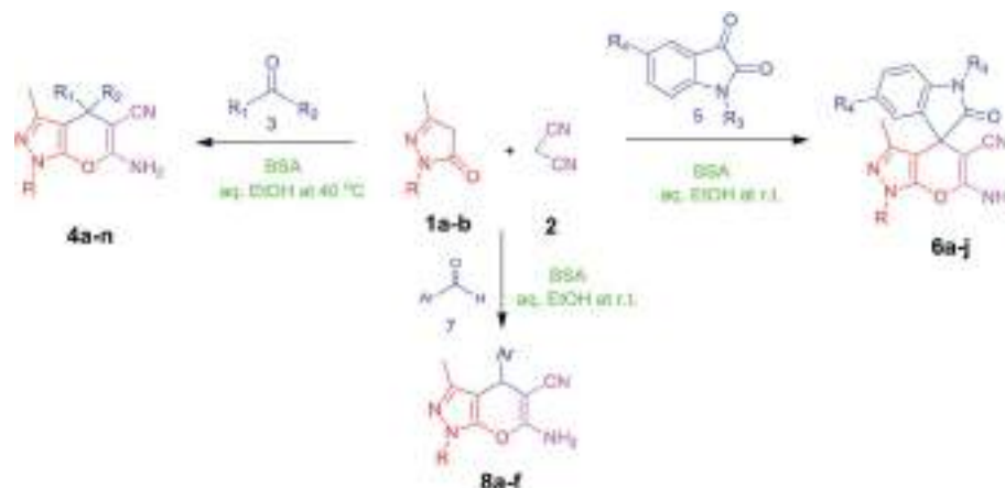
Scheme 1 Synthesis of dihydropyrano[2,3-c]pyrazoles and spiro[indoline-3,4'-pyrano[2,3-c]pyrazoles in aqueous ethanol.
